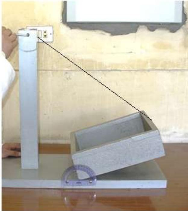
**Fig. (1) Static Friction Coefficient Measurement Apparatus.**
